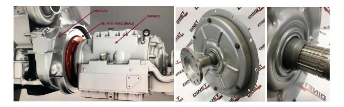
In the buses equipped with Voith gearboxes, for example, the Torsional Damper is connected (by screws) to the engine flywheel with its outer casing flange and to the gearbox Input Shaft through the slotted central hub.
